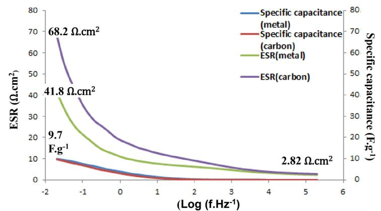
Figure 4: Bode plot of two type of devices from 10 kHz to 20 mHz, extract from EIS test with equivalent series resistance (ESR) marked
