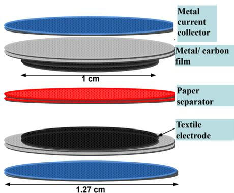
Figure 3: cross-sectional view of testing setup with fabric electrode on metal foil and steel corrector
