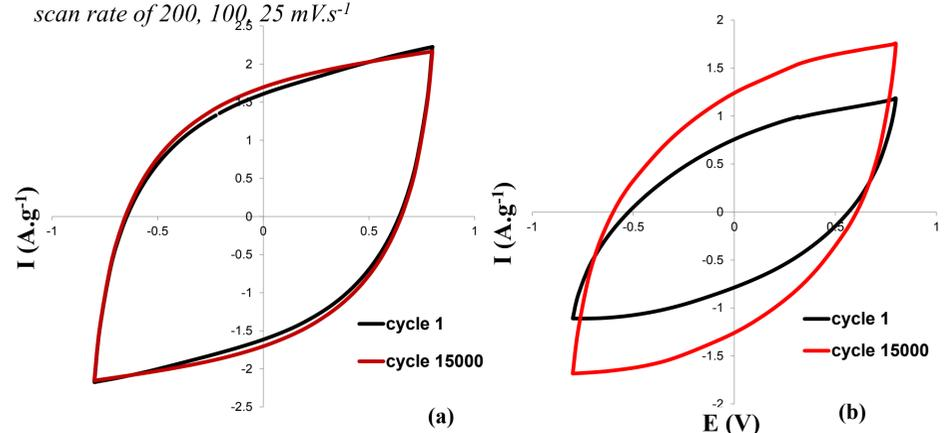
Figure 6: CV test of the device for 15000 cycles between +/- 0.8 V at the scan rate of  $200 \text{ mV}\cdot\text{s}^{-1}$  (a) metal encapsulated supercapacitor, (b) carbon film encapsulated supercapacitor
