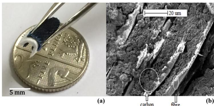
Figure 1. (a) wearable carbon fabric and paper separator (b): SEM images of fabric electrode
