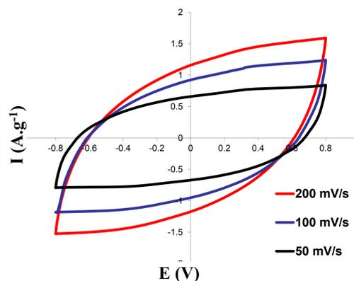
Figure 5: CV test of the carbon film encapsulated device between +/- 0.8 V at the scan rate of 200, 100, 25  $\text{mV}\cdot\text{s}^{-1}$
